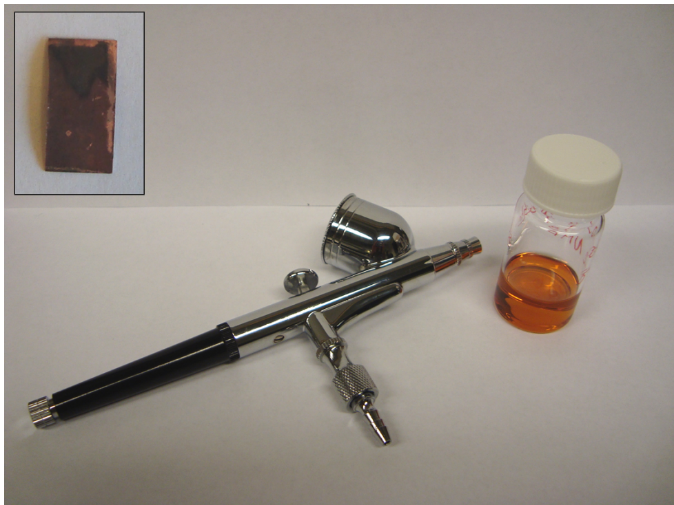
Figure S7. Photo of the airbrush pen and the iron acetate solution used for aerosol generation and infiltration of the as-electrodeposited 3D current collector. The inset is a photo showing the 3D current collector after the infiltration and pyrolysis processes.
