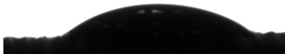
Figure S4. PEM carrying chloride counterions exhibits hydrophilicity with a WCA of 35°.
