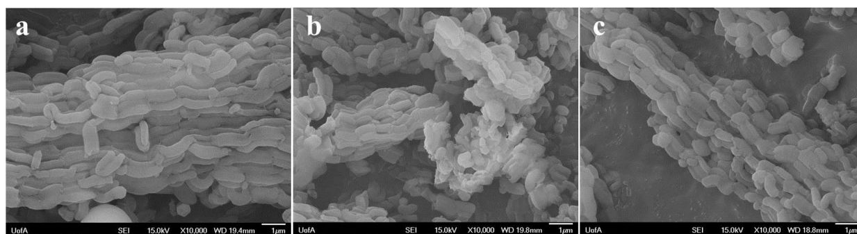
Figure S2. SEM images of (a) SBA-15, (b) SBA-15-5% Ag, (c) SBA-15-10% Ag when using silver ammonia solution as the Ag source.
