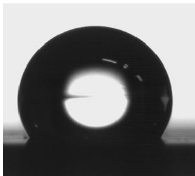
Fig. S1. Water profile on the as-prepared SU-8 void array. The water contact angle is 120^\circ .
