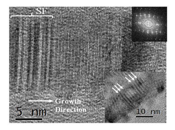
**Fig. S1** HRTEM image of S3 sample at two different magnification showing the presence of stacking faults.
