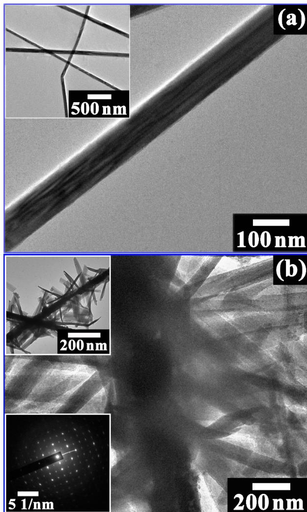
**S2:** TEM images of (a) Cu nanowire (inset shows the low magnification image); (b) T5 (upper inset for T2) and SAED of T5 in the lower inset.
