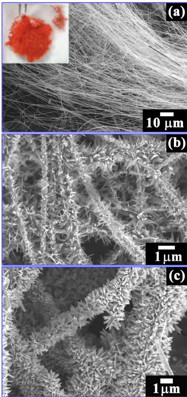
**S1:** FESEM images of (a) Cu nanowires (inset showing digital image); (b) CuTCNQ nano-hierarchy (T2) and (c) CuTCNQ nano-garland (T5) showing scalability.
