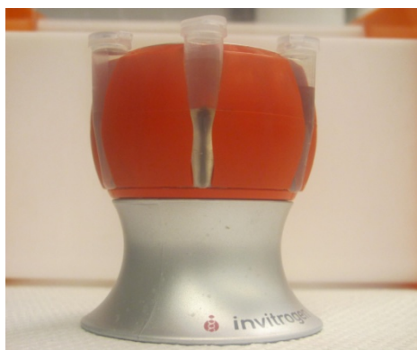
Figure S3. Demonstration of magnetic property of the Ag-Fe 3 O 4 nanocomposites.
