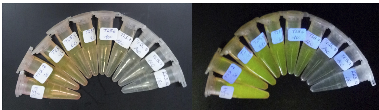
Figure S9. Photographs of the different samples taken along the degradation reaction of an aqueous solution of Rhodamine 6G ( 5 \cdot 10^{-5} M) under UV light irradiation using as photocatalysts TiO 2 -PPD-b (left visible illumination, right UV illumination).
