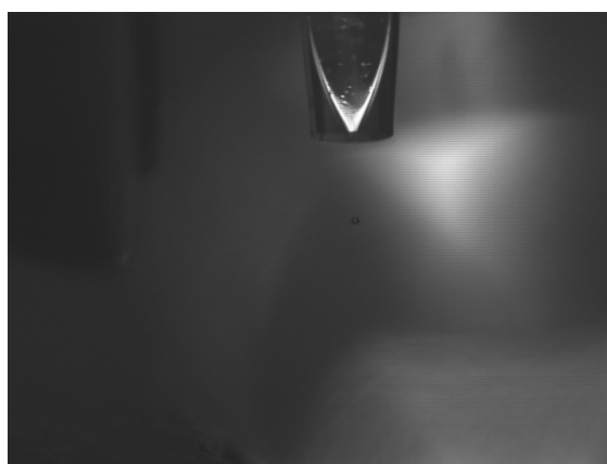
Figure S8. The photograph of a piezoelectric inkjet print head during inkjet printing, which demonstrates the excellent stability of the ink droplet.
