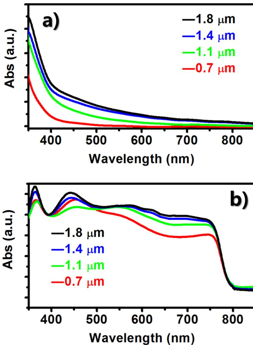
**Figure S4** UV-vis absorption spectra for a) FTO/TiO<sub>2</sub> NRs and b) FTO/TiO<sub>2</sub> NRs/CH<sub>3</sub>NH<sub>3</sub>PbI<sub>3</sub> with different NR film thickness.
