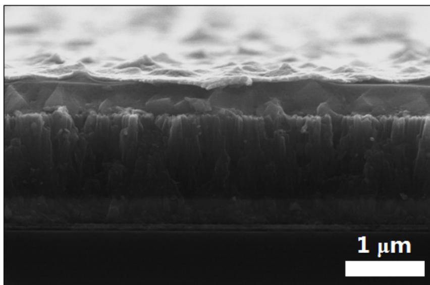
**Figure S2** Cross-sectional SEM image of a perovskite solar cell device based on ~ 1.1 μm TiO<sub>2</sub> NR film.
