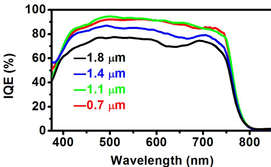
**Figure S5** Internal quantum efficiency (IQE) spectrum for the perovskite solar cells base on different NR film thickness.
