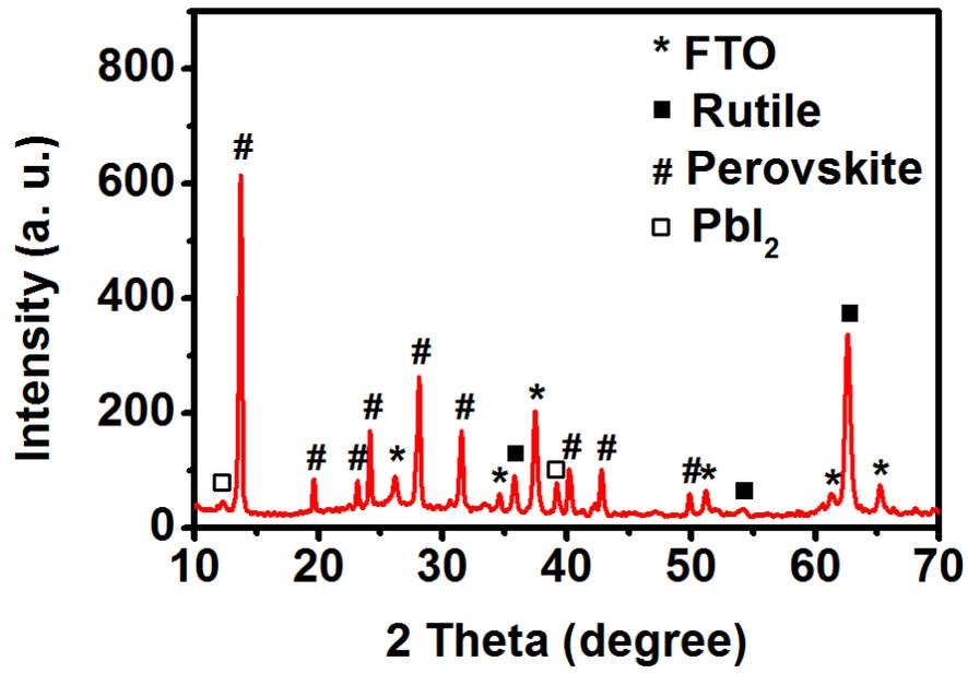
Figure S3 XRD pattern for the sample of  $\sim 1.1 \mu\text{m}$   $\text{TiO}_2$  NRs/  $\text{CH}_3\text{NH}_3\text{PbI}_3$
