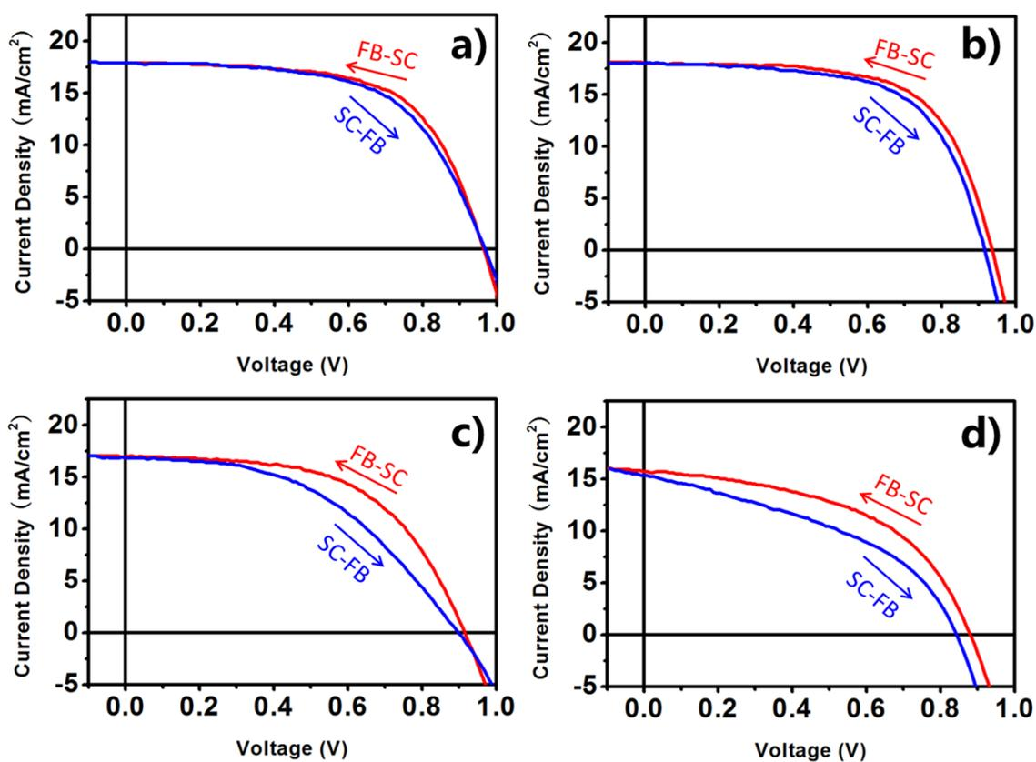
**Figure S6** The J-V hysteresis depending on NR thickness: a) 0.7  $\mu\text{m}$ , b) 1.1  $\mu\text{m}$ , c) 1.4  $\mu\text{m}$  and d) 1.8  $\mu\text{m}$ . The device was scanned from forward bias to short circuit (FB-SC, red) and from short circuit to forward (SC-FB, blue) under simulated AM1.5G solar irradiation of 100  $\text{mW}/\text{cm}^2$  with a scan rate of  $\sim 0.1$  V/s.
