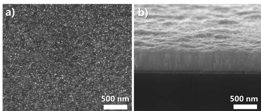
**Figure S1** SEM images of TiO<sub>2</sub> nanoparticles synthesized with 25 mM Na<sub>2</sub>EDTA, 33.0 mM TTIP (10.0 μl/ml aqueous solution), 2.5 vol.% glycerol in aqueous solution and growth time 3 h.
